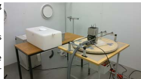
Figure 2: Equipment used for generation of sanding dust at NRCWE.
